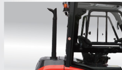
Upward Exhaust Pipe I
